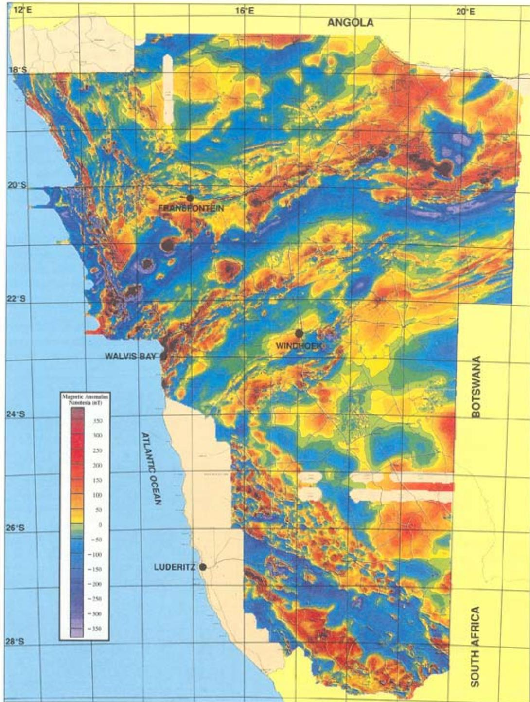
Figure 3: The airborne magnetic anomaly map of Namibia, in nT, with the International Geomagnetic Reference Field (IGRF) at time of data acquisition subtracted.
