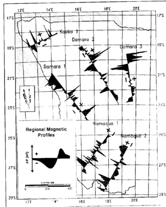
Figure 7: Location of six regional magnetic profiles interpolated from the airborne magnetic gridded data (cell size 2 000 m).
