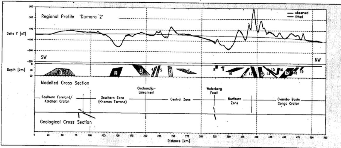
**Figure 8:** Regional magnetic profile 'Damara 2' extending from the Gobabis area in the southeast to the Etosha Pan in the northwest, with simplified geological cross section. The parameters of the modelled source bodies are given in Table 2.
